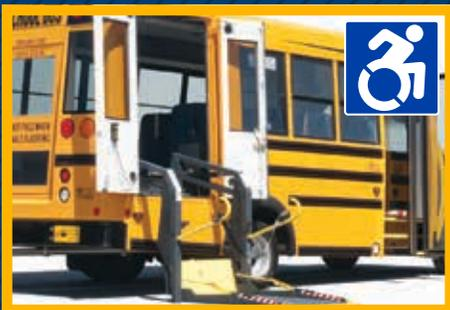
Special needs Micro Bird with double-leaf wheelchair doors offer protection on both sides of the lift, thus adding to passenger safety, while offering superior weather seal and door strength.
