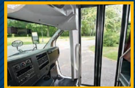
Maximum visibility of loading zone is provided by fully-glassed entrance door and unobstructed "More-View" window. Standard 32" electric double-opening door.
