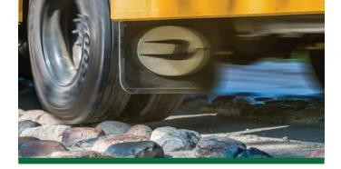
Blue Bird performs full vehicle accelerated durability testing that approximates 300,000 miles service life of the vehicle at an automotive proving ground. This rigorous evaluation includes cobblestones, inverted chatter bumps, impact bumps, undulated road, staggered bumps for chassis torsion and resonance road.
