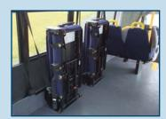
Folding seats maximize flexibility of configurations by using the same space for either seated passengers or wheelchair locations.
