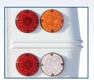
LED clearance lights, direction lights, stop lights and back-up lights are standard equipment offering enhanced safety, while reducing operating and maintenance costs.
