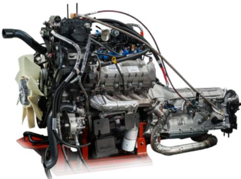
The Ford 6R140 Transmission, **exclusive to our Propane and Gasoline Vision buses**, is capable of increasing torque demand in many vehicle applications – it is purpose built to exact torque requirements to achieve minimal friction losses. This results in **best possible fuel economy** to all customers. Fluid change interval is 150,000 miles. The proven powertrain combination of the Ford 6.8L engine and Ford 6R140 transmission comes with a **standard 5-year, unlimited mile warranty**.
