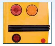
LED clearance lights, direction lights and stop lights are standard equipment offering enhanced safety, while reducing operating and maintenance costs.
