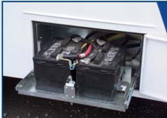
An optional fully-enclosed battery box with stainless steel hinge and galvanized steel tray on roller bearings is available for added convenience and protection from the elements.
