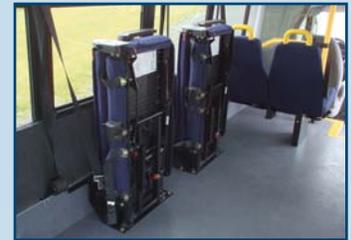
Folding seats maximize flexibility of configurations by using the same space for either seated passengers or wheelchair locations.
