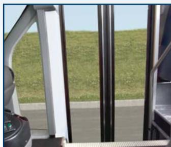
Maximum visibility of the loading zone is provided by a fully-glassed entrance door and unobstructed "More-View" window.
